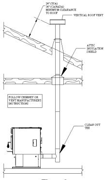
Figure 9 Venting through roof
